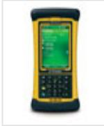
The Trimble Nomad 900 Series rugged handheld computer packs functionality into one of the most powerful and full-featured rugged handheld PCs available. The Nomad meets demanding military standards for drops, vibration, humidity, altitude, and temperature extremes. It also comes with an IP68 rating, meaning the Nomad handheld PC is completely sealed against dust, and can survive immersion in up to a meter of water for 240 minutes. This rugged handheld computer is truly ready for the outdoors!
